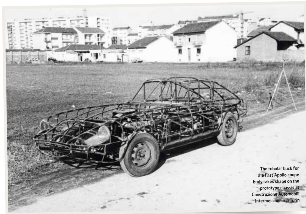
The tubular buck for the first Apollo coupe body takes shape on the prototype chassis at Construzione Automobili Intermecanica in Turin
